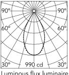
Luminous flux luminaire 704 lm (EXTREME CUT OFF)
