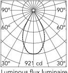
Luminous flux luminaire 723 lm (EXTREME CUT OFF)
