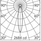
Luminous flux luminaire 710 lm (EXTREME CUT OFF)
