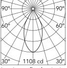
Luminous flux luminaire 715 lm (EXTREME CUT OFF)
