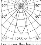
Luminous flux luminaire 687 lm (EXTREME CUT OFF)
