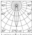
Luminous flux luminaire 739 lm (EXTREME CUT OFF)
