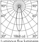
Luminous flux luminaire 630 lm (EXTREME CUT OFF)
