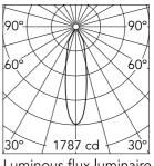
Luminous flux luminaire 541 lm (EXTREME CUT OFF)
