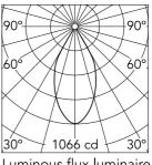
Luminous flux luminaire 688 lm (EXTREME CUT OFF)
