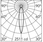
Luminous flux luminaire 667 lm (EXTREME CUT OFF)
