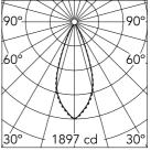
Luminous flux luminaire 882 lm (EXTREME CUT OFF)
