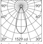
Luminous flux luminaire 703 lm (EXTREME CUT OFF)
