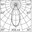
Luminous flux luminaire 995 lm (EXTREME CUT OFF)
