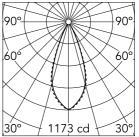
Luminous flux luminaire 585 lm (EXTREME CUT OFF)
