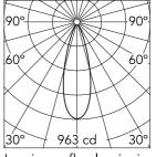
Luminous flux luminaire (EXTREME CUT OFF)
