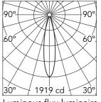
Luminous flux luminaire 359 lm (EXTREME CUT OFF)
