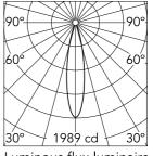
Luminous flux luminaire (EXTREME CUT OFF)
