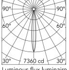
Luminous flux luminaire 385 lm (EXTREME CUT OFF)
