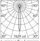
Luminous flux luminaire 399 lm (EXTREME CUT OFF)
