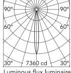
Luminous flux luminaire 385 lm (EXTREME CUT OFF)
