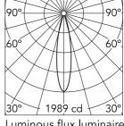
Luminous flux luminaire 373 lm (EXTREME CUT OFF)
