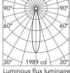
Luminous flux luminaire 373 lm (EXTREME CUT OFF)
