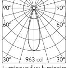
Luminous flux luminaire 300 lm (EXTREME CUT OFF)
