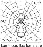
Luminous flux luminaire 8356 lm
