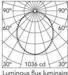
Luminous flux luminaire 2733 lm
