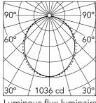
Luminous flux luminaire 2733 lm
