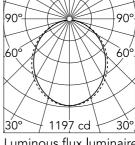
Luminous flux luminaire 3155 lm
