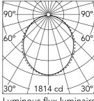
Luminous flux luminaire 4783 lm
