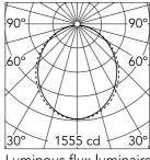
Luminous flux luminaire 4100 lm
