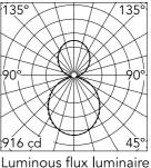
Luminous flux luminaire 4036 lm
