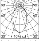
Luminous flux luminaire 1660 lm
