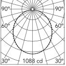
Luminous flux luminaire 2958 lm
