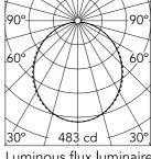
Beam Angle: 107° h(m)  $E(I_X)$ D(m) 483 2.63 2 5.26 121 3 54 7.90 4 30 10.53 5 19 13.16
