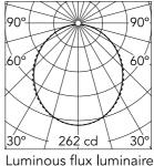
Beam Angle: 107° h(m)  $E(I_X)$ D(m) 262 2.63 2 65 5.26 3 29 7.90 4 16 10.53 5 10 13.16
