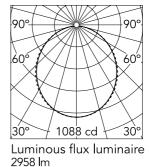
Beam Angle: 107° h(m) E(Ix)D(m) 1088 2.63 2 5.26 272 3 121 7.90 4 68 10.53 5 44 13.16
