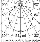
Luminous flux luminaire 2301 lm
