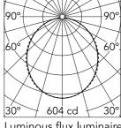
Beam Angle: 107° h(m)  $E(I_X)$ D(m) 604 2.63 2 5.26 151 3 67 7.90 4 38 10.53 5 24 13.16
