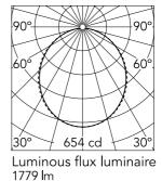
Beam Angle: 107° h(m)  $E(I_X)$ D(m) 654 2.63 2 164 5.26 3 73 7.90 4 41 10.53 5 26 13.16
