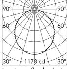
Luminous flux luminaire 3203 lm
