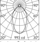
Luminous flux luminaire 1534 lm
