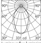
Luminous flux luminaire 511 lm
