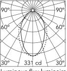
Luminous flux luminaire 511 lm
