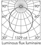
Beam Angle: 107° h(m) E(Ix)D(m) 1329 2.63 2 332 5.26 3 148 7.90 4 83 10.53 5 53 13.16
