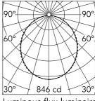
Luminous flux luminaire 2301 lm
