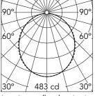
Luminous flux luminaire 1315 lm
