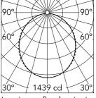
Beam Angle: 107° h(m) E(Ix)D(m) 1439 2.63 2 360 5.26 3 160 7.90 90 10.53 5 58 13.16
