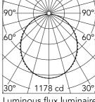
Luminous flux luminaire 3203 lm
