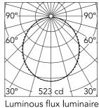
Beam Angle: 107°  $E(I_X)$ D(m) h(m) 523 2.63 2 131 5.26 3 58 7.90 4 33 10.53 5 21 13.16
