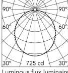
Beam Angle: 107° h(m)  $E(I_X)$ D(m) 725 2.63 2 181 5.26 3 81 7.90 4 45 10.53 5 29 13.16
