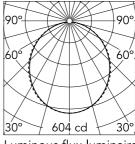
Luminous flux luminaire 1643 lm
